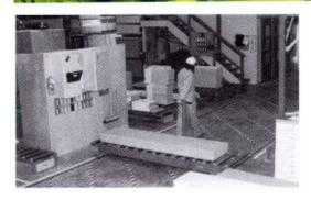
Panels are moved effortlessly through the plant and to the second floor mezzanine on a series of roller conveyors and lifts.
